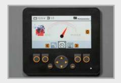
Machine performance management (optional) allows adjustment of engine power as needed. This can save fuel or provide extra power.
