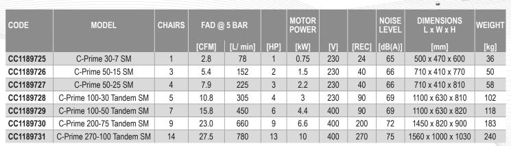
Models can be configurated to 10 Bar maximum pressure offering on average 33% lower FAD @ 8 Bar
