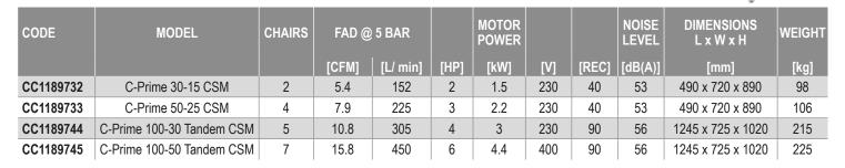
Models can be configurated to 10 Bar maximum pressure offering on average 33% lower FAD @ 8 Bar
