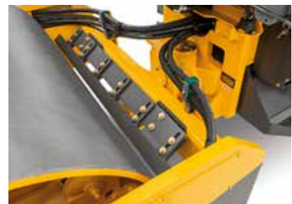
Inside drum scraper
